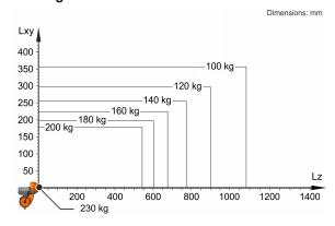
The KR 180 R3200-2 PA is designed for a rated payload of 180 kg in order to optimize the dynamic performance of the robot. With reduced load center distances and favorable supplementary loads, a maximum payload of up to 230 kg can be mounted. The specific KUKA Load case must be verified using KUKA. For further consultation, please contact KUKA Service.
