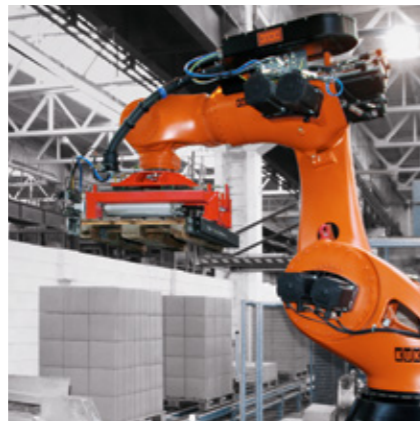
Handling of concrete blocks with the KR 1000 titan
