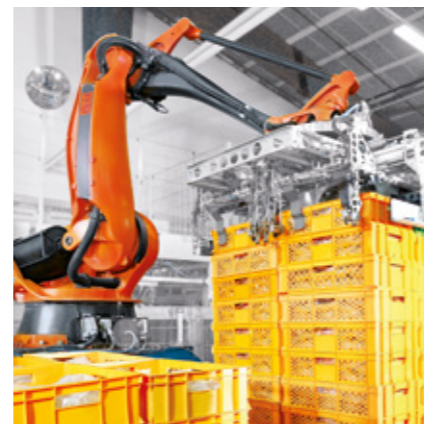
Palletizing of bread crates with the KR 180 PA
