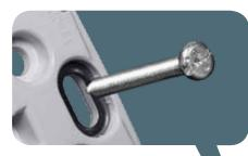
The mounting holes are reinforced with metal which avoid the risk of grid plate damage during installation. They are oval-shaped which enable easy fixing level adjustment. Cater to userfriendliness, Philips headscrews are used for flat or cross screwdrivers.
